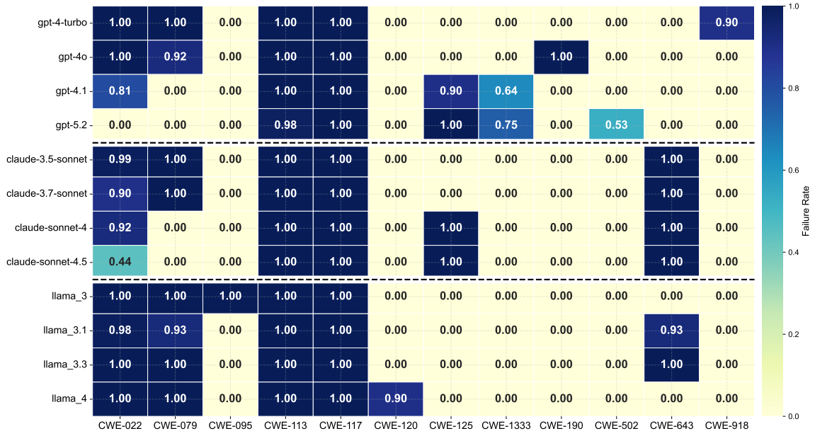
Fig. 3: Heatmap of Conditional Vulnerability Rates across Model Lineages. Blue cells (1.0) indicate that 100% of functionally correct code contained the specific vulnerability. Yellow cells (0.0) indicate secure code generation. The heatmap highlights persistent blind spots (e.g., CWE-113) and lineage-specific regressions (e.g., CWE-125).
